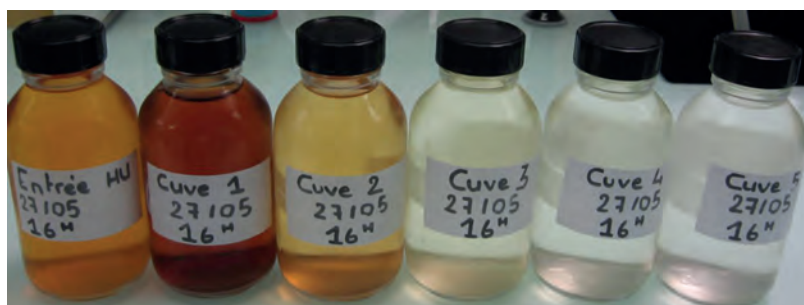
Figure 14: Samples during treatment by UV oxidation; from left to right: untreated wastewater to final treated wastewater.
