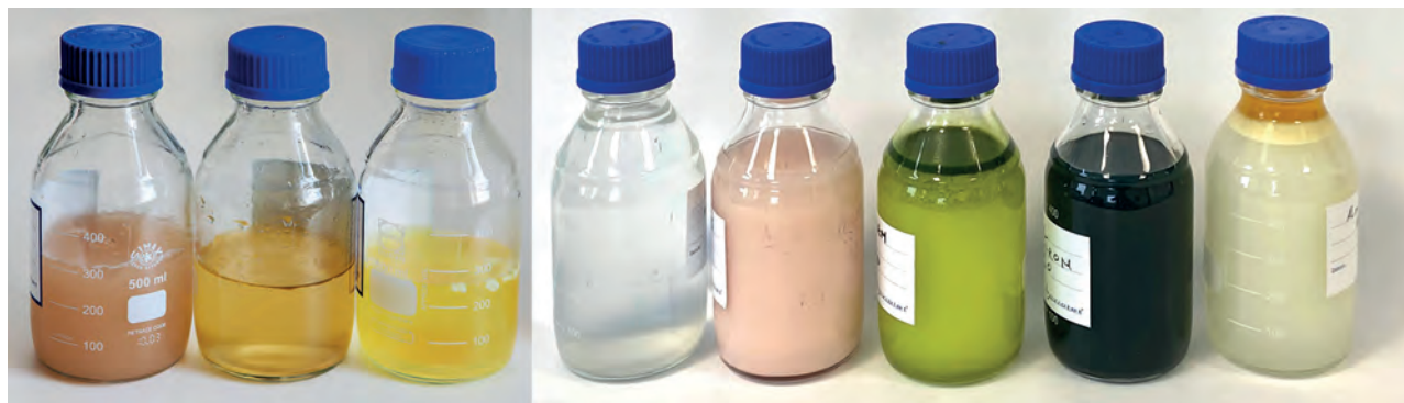
Figure 1: Examples of different pharmaceutical Cleaning-in-Place (CIP) rinse wastewater samples (untreated) (source of all figures: the authors).
