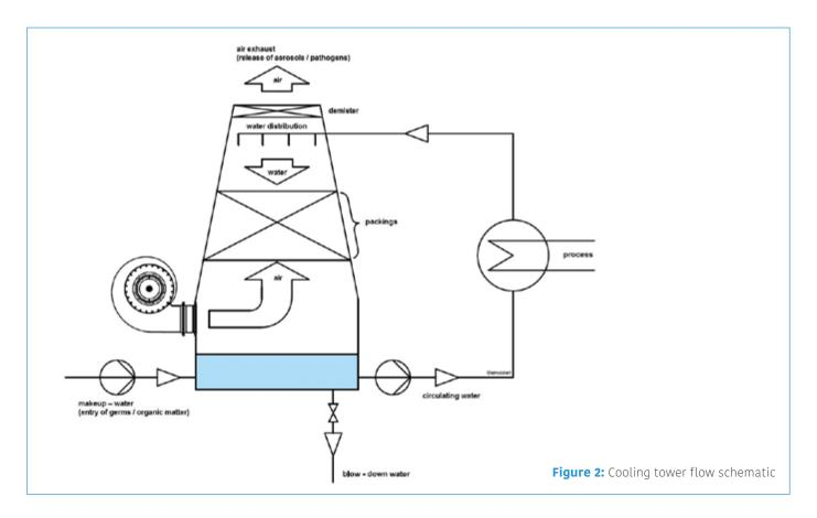
enthalpy is generating a cooling effect on the remaining water within the system (**Figure 2**).
