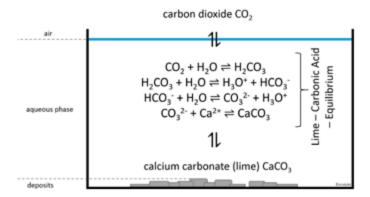
**Figure 4:** Schematic illustration of the calcium carbonate-carbonic acid-equilibrium
