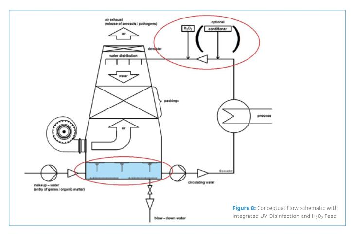
of the UV-lamps in the cooling tower tank or other auxiliary tanks, there are assorted, legally protected systems available:
