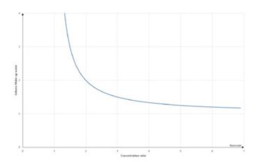
**Figure 3:** Fresh water demand with increasing concentration (recirculating water volume constant)
