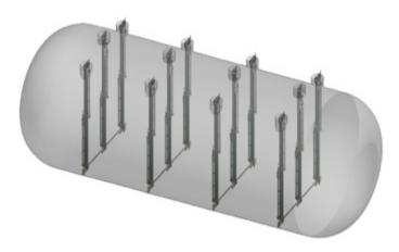
**Figure 7:** Example of mounting bracket systems for submerged UV-lamps in KTC-tanks
