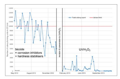
**Figure 9:** Bacteria growth, total bacteria count/ year (GKZ), KBE/ml = Colony Building Units per ml (prior to UV-H<sub>2</sub>O<sub>2</sub> system installation of a biologic strongly affected cooling tower)
