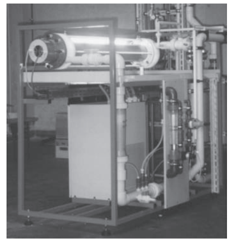
Figure 1. Enviolet® 12 UV-Reactor with process technology for optimal process requirements: In the UV-facility all necessary systems for process control and safety, also the dosing and mixing of the chemicals are fully integrated. The performance transformers of the systems are located near the reactor and are monitoring the optimal performance through a patented process.
